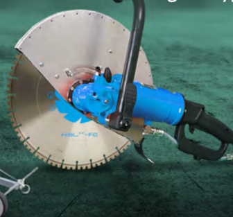
Tyrolit TS40 Precut Steinsög - rafknúin Sögunardýpt 16,5cm
